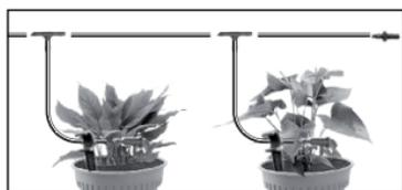
**C** Cut the tube to desired length, connect it with drippers by a barbed tee, and fix the drippers by tube holder stakes
