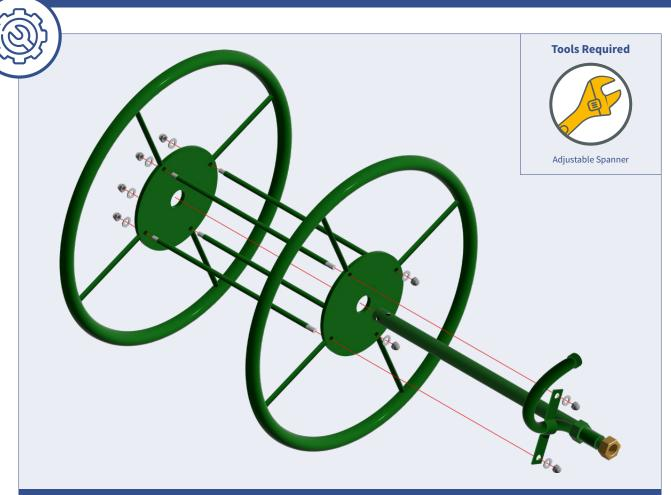
Insert the ends of four Rods (B) into one Spool (A) and secure with Ø8 Washers and M8 Nuts. Insert the opposite ends of the four Rods (B) into the remaining Spool (A) and secure just two of the Rods with Ø8 Washers and M8 Nuts, leaving two adjacent ends open.
