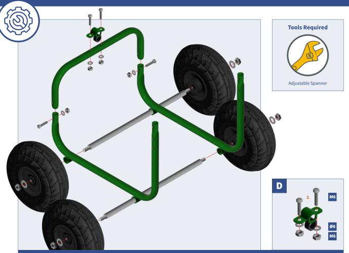
Slide two Axles (E3) into the holes of both Axle Bracket Frames (E1) and attach a Wheel to the end of each Axle. Secure the wheels with Ø12 Washers & M12 Nuts. Slot the U-Shape Frame (E2) onto the short end of the Axle Bracket Frame (E1) and secure with M6 Bolts, Ø6 Washers & M6 Nuts.
