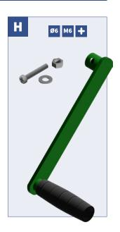
Slide the Winder Handle (H) onto the Axle Shaft. Secure with M6 Screw, Ø6 Washer and M6 Nut (H) using the Adjustable Spanner and Cross head Screwdriver.
