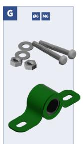
At the Rear of the Cart above Axle (B). The Drum Shaft will be resting on top of the Frame. Slide Bearing Bracket (G) onto the Drum Shaft and Align with the Two Holes on the Frame. Secure with M6 Bolts, Ø6 Washers and M6 Nuts (G).
