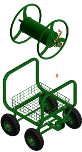
Place Assembled Hose Drum (F) onto the Frame.
