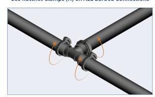
Pinch Ratchet Clamps & check for leaks
