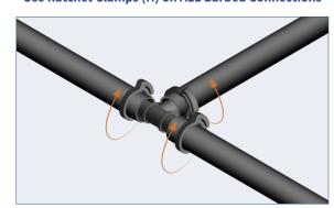
**Pinch Ratchet Clamps & check for leaks**
