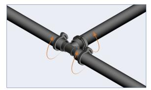
Pinch Ratchet Clamps & check for leaks
